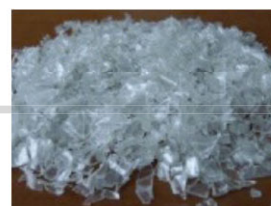
Melted and grained into PET chips
