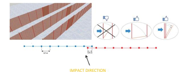
The "Uphill" group (red) should surmount the "Downhill" one (blue), to avoid that the fallen skier can impact and pass through the only opening of the net, at the joint by two net groups.
