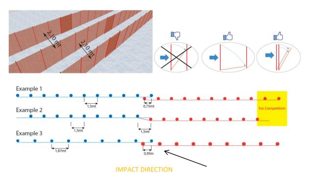
The "Uphill" group (red) should surmount at the "Downhill" one (blue), to avoid that the fallen skier can impact and pass through the only opening of the net, at the joint by two net groups.
